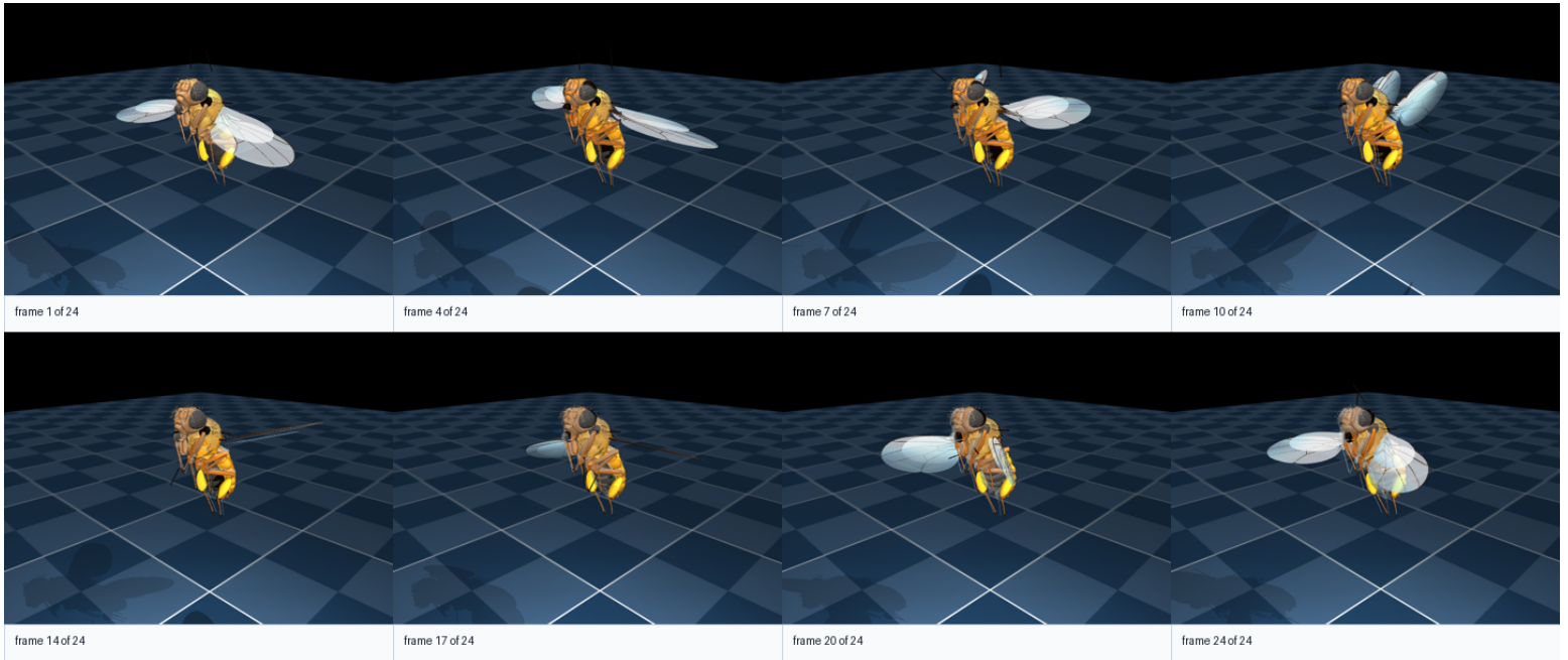
Figure 5: FlyBody/MuJoCo beebody flybody wing-beat flight render shows Eight-frame contact sheet from FlightImitationWBPG and WingBeatPatternGenerator on the same honeybee MJCF, showing coupled forewing/hindwing surfaces and wing-beat flight posture. Generated from animation manifest, bee visual verification, and apis mellifera worker MJCF. Sidecar validation checks raster, source routing, and registered claim tier. Does not calibrate honeybee aerodynamics or hovering power against measured loads.
